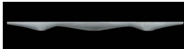
Figure 2.18: Concrete beam made with fabric formwork
